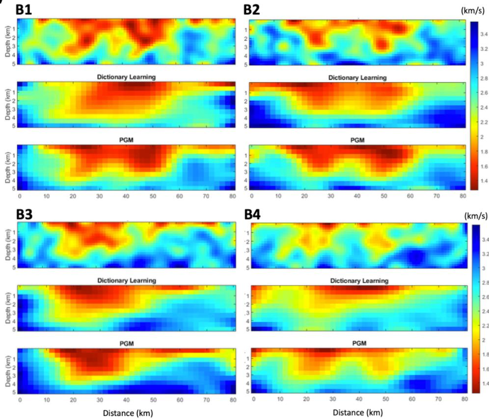
Figure 1: (a) Station locations (triangles) and main faults (lines) surrounding the Ridgecrest area. There are six dense sensor arrays across the main faults (A1-2 and B1-4). (b) Vertical cross-sections of the shear wave velocity along the B1-4 station arrays from (top) surface wave dispersion inversion, (center) the 3D fusion model from dictionary learning, and (bottom) the PGM.
