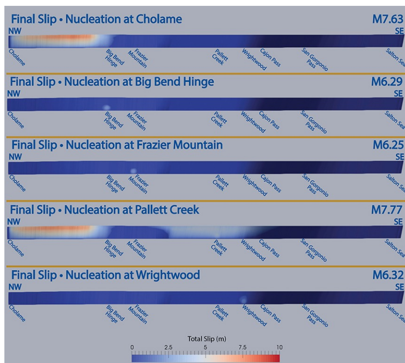
Figure 1. Slip distributions from preliminary dynamic rupture simulations in the vicinity of the Big Bend of the San Andreas Fault. Notice that, regardless of nucleation point, none of these ruptures propagate around the bend.
